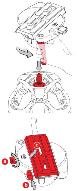
Hold the adaptor firmly with both hands. Pull the lever all the way back towards the level bubble.
