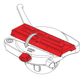
Place the camera plate with the slider fitted into the dovetail and lower into place.
