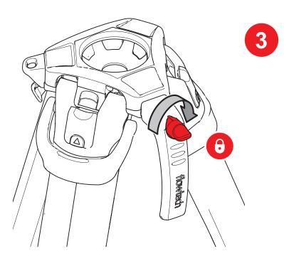
To place the handle back into the carry position: Rotate the handle back into the lock position and tighten the Lock Knob.
