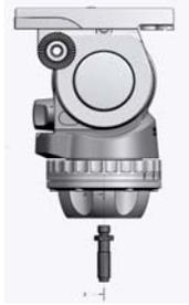
If you want to fit the FSB 6 onto on a flat base, remove the threaded pin.
